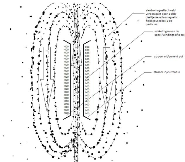
Field lines can be made clear when using iron filings randomly dropped on paper that is covering the magnet. When you shake the paper in a gently way the field pattern will occur.
