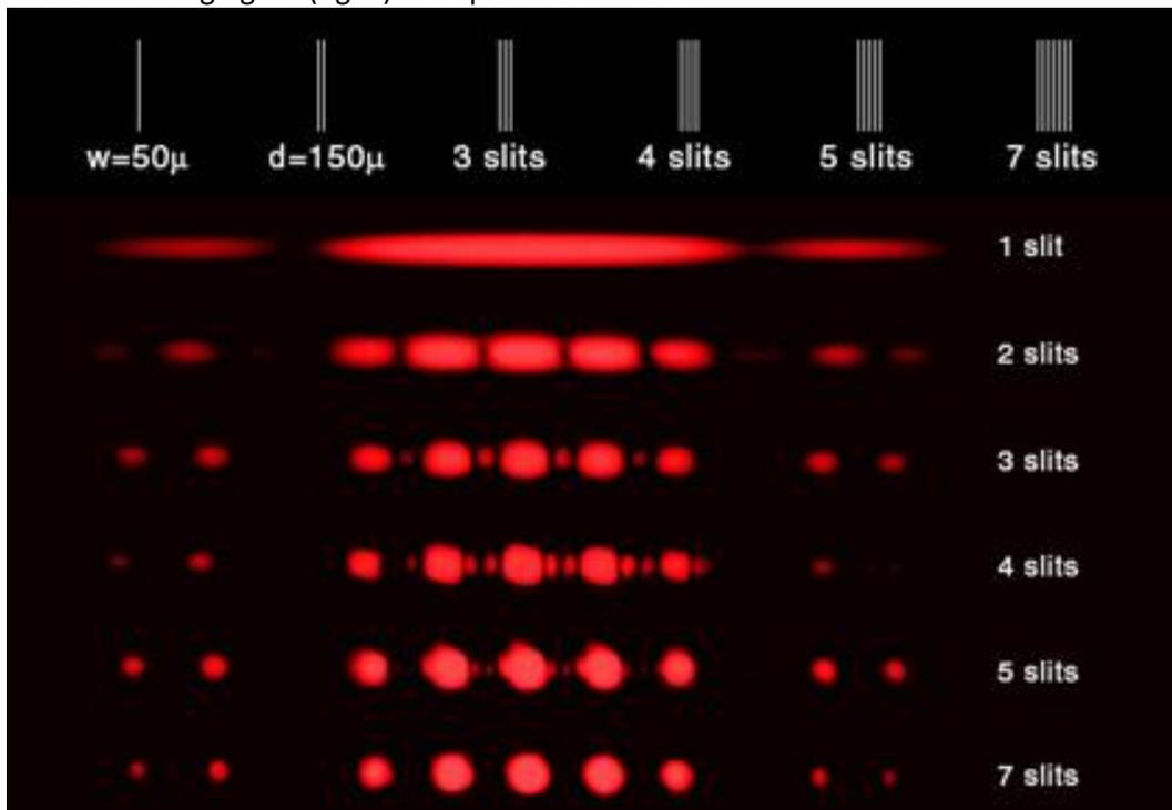
Fig. 3 The effect of multiple slits /aluminium slide
